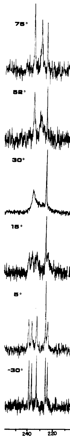
Figure 2. Variable-temperature ^{13}\text{C} NMR spectra (carbonyl region) of \text{Mn}_2(\text{CO})_5(\text{dpm})_2 under conditions of broad-band ^{31}\text{P} decoupling.
